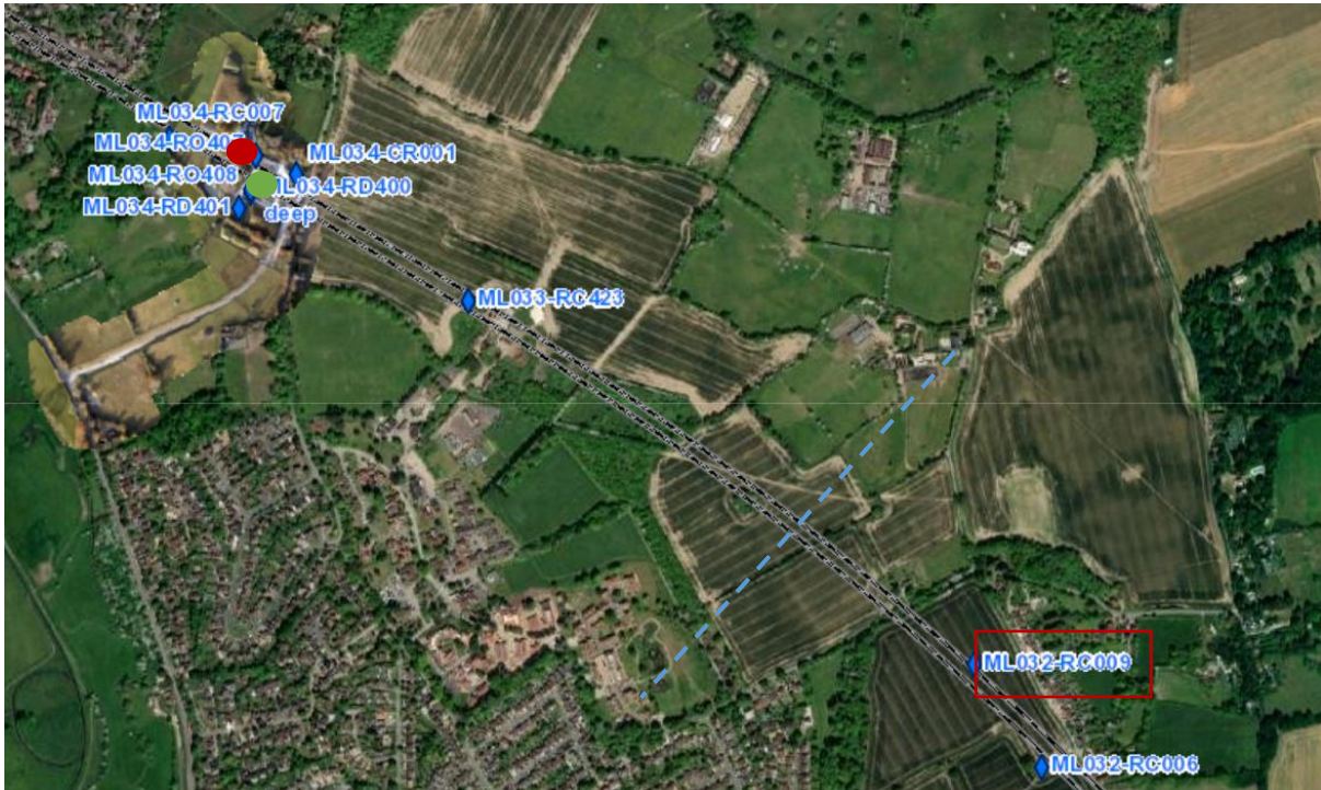
Figure 2 Location of TBMs in early Nov 2021 in relation to monitoring boreholes (ML032-RC009 outlined in red)
